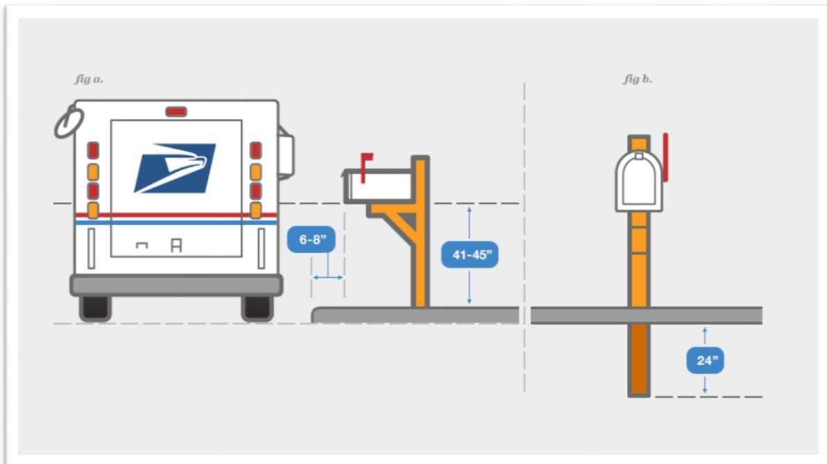
Minimum depth for setting post is 24" (using poured concrete to secure). Position your mailbox 41-45" from the road surface to the bottom of the mailbox. Set your mailbox 6-8" back from the curb.
